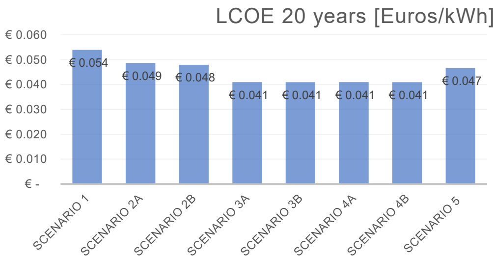
Figure 4: Preliminary results of the LCOE analysis for various SYMBIOSYST scenarios for PV module layout and mounting structures
