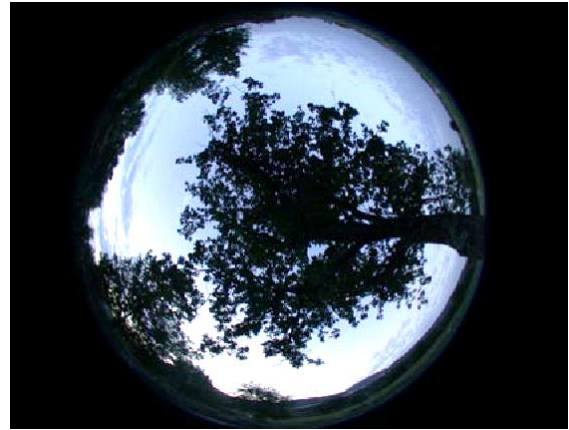
Figure 1: Illustration depicting the concept of optical porosity, which represents the fraction of sunlight that is transmitted through a canopy [6].
