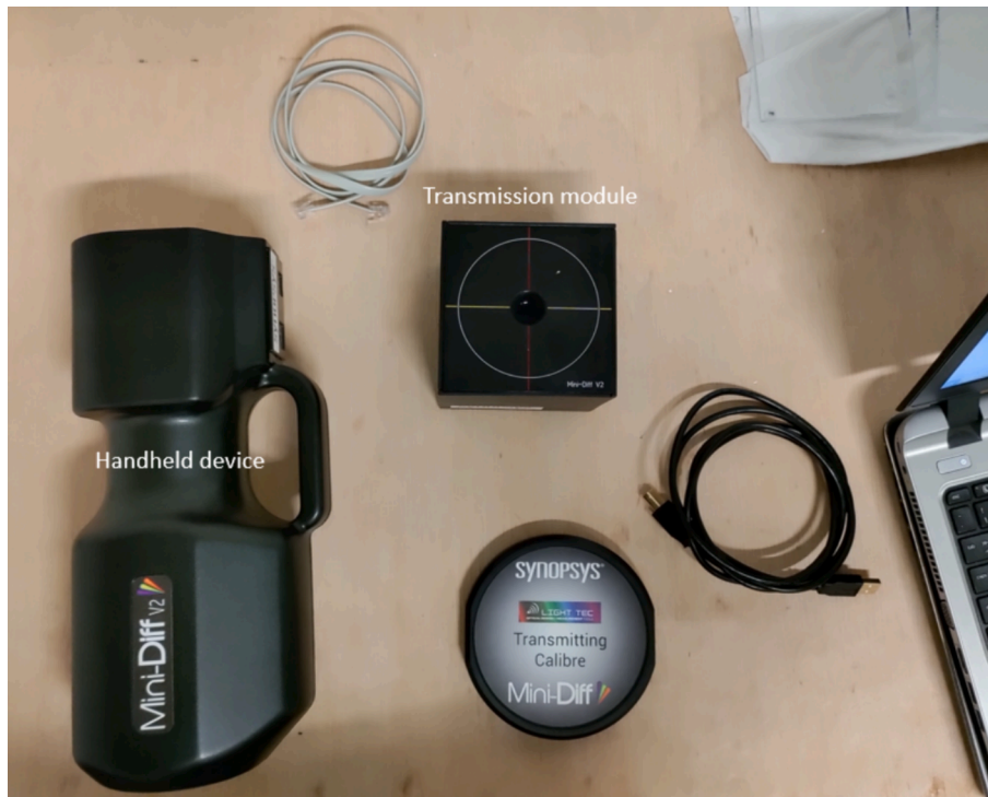
Fig. 5. Picture of the Mini-Diff V2 from Synopsys and its schematics. The handheld device has 4 collimated LEDs, one for each AOI, namely 0^\circ , 20^\circ , 40^\circ , and 60^\circ . Three of the LEDs each has a single emission peak at wavelengths of 465 nm, 525 nm, and 630 nm and are focused on the lower part of it. The diffusely reflected light of the probed surface at its bottom is collected and detected by a camera situated on top allowing for BRDF measurements. For transmission measurements, a transmission module with 4 other LEDs allows the camera to capture the BTDF for the same configuration as with the handheld device.
