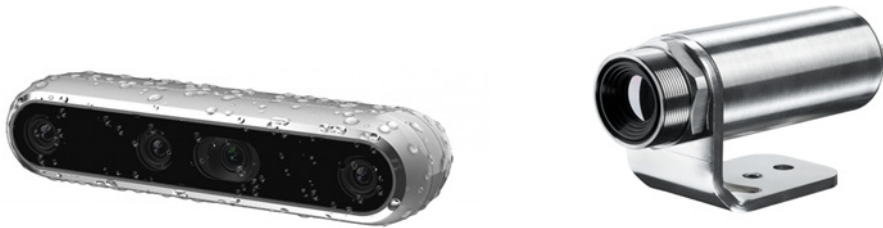
Figure 16: Intel RealSense D457 RGB Camera (left); Optris Xi 400 Thermal Camera (right).
